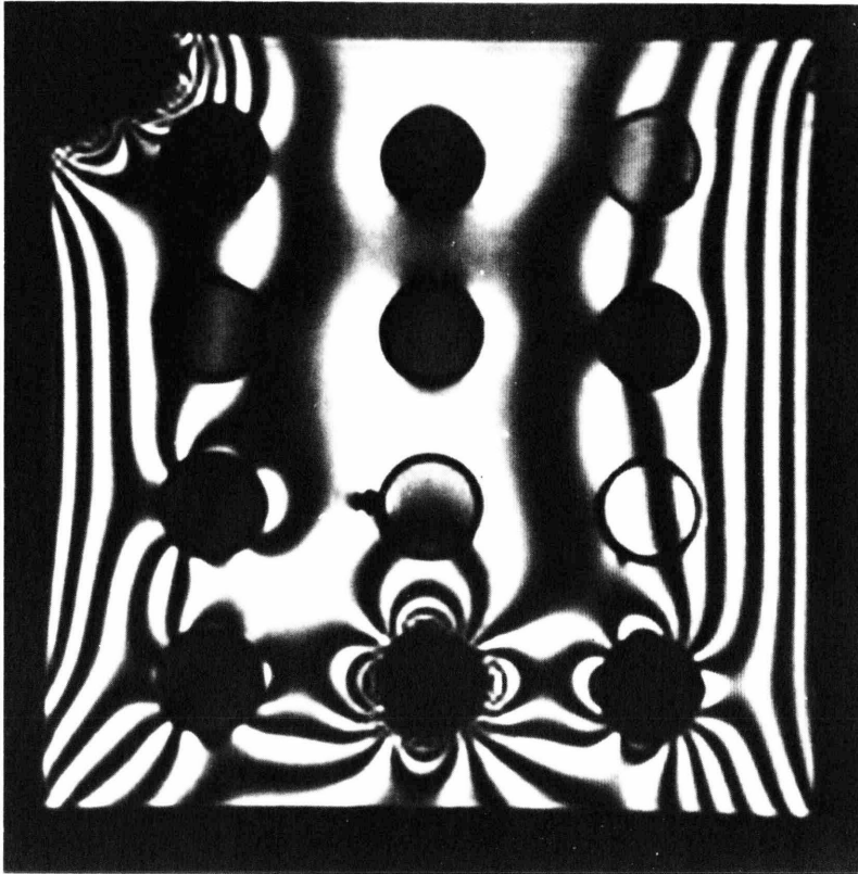
Fig. 7. Two-pulse SENEX sequence applied to a relaxation phantom containing vessels with different amounts of GdDTPA. The characteristics of the frequency selective excitation are visible as contour plots superimposed to the NMR image. Clearly the image plus the magnetic field behaviour, changed by the object itself, can be recorded. – Slice thickness : 10 mm, matrix size : 256 \times 256 , measuring time : 4.27 min., frequency difference between two dark structures : 32 Hz that means 0.5 ppm.
